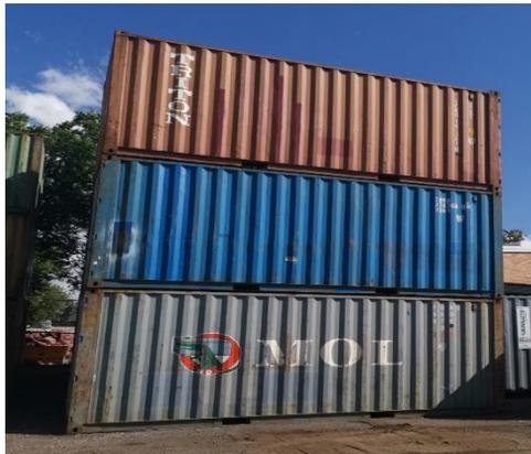
Shipping containers have **durable strength** suitable to **withstand shipment, storage, and handling**. All container **sizes are standardized** across the global industry to provide stacked shipping efficiency. Shipping containers are constructed out of **steel**, where all containers sizes and types are built according to the same ISO specifications, regardless of where the container is manufactured.
